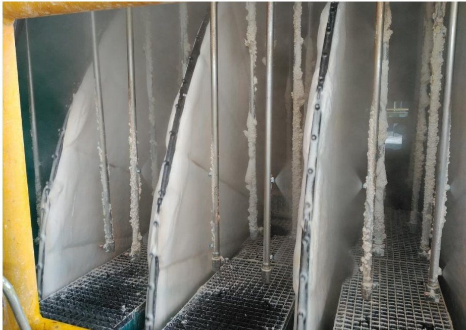
Figure 3. BoVac Disc Filter for Al-hydrate filtration with cake wash
