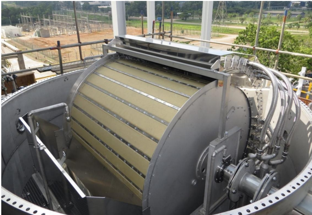
Figure 2. BoHiBar Drum Filter with open pressure vessel for purified terephthalic acid (PTA) filtration
